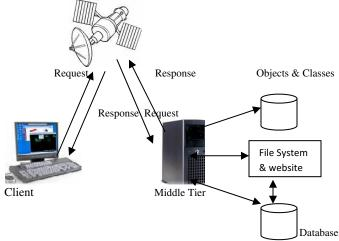
Figure 3: Three-Tier Architecture
